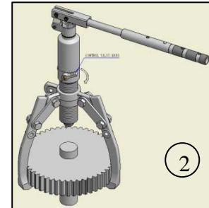
**IMPORTANT ! position the control valve knob so it does not contact the puller head and can be turned freely. See Figure 2.**
